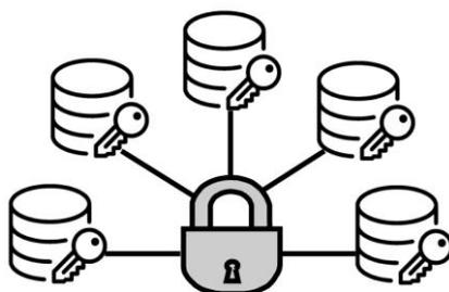
Multiple IBM i LPARs using single IBM i Key Manager
